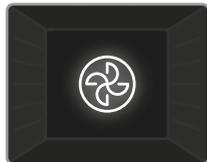
**Turbo Function:** The oven's thermostat and warning lights will switch on, and the ring heating element and fan will start operating. The turbo function evenly disperses the heat in the oven so all food on all racks will cook evenly. It is recommended that you preheat the oven for about 10 minutes.
