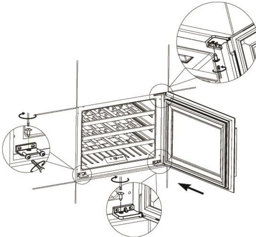
1. Put the wine cooler into the cabinet, then adjust the wine cooler to make it steady. Open the door, take out the fixed plate, 2pcs Inner Hexagon Screws, and Inner Hexagon Screwdriver from accessory bag, then use the inner hexagon screwdriver to tighten the fixed plate on the lower left side of wine cooler.
