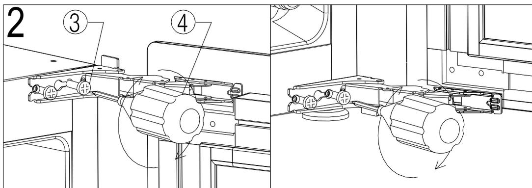
4. Rotate the door by 180 degrees, and install it to the other side of the cabinet. (Figure 3 and 4)
