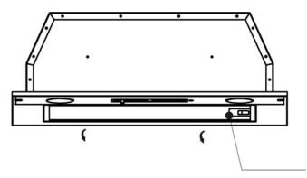
• Activated carbon filter can be used to trap odors. In order to install the activated carbon filter, unscrew and take down the front panel. Then plug the activated carbon filter into the unit and turn it in anti-clockwise. Repeat the same on the other side.
