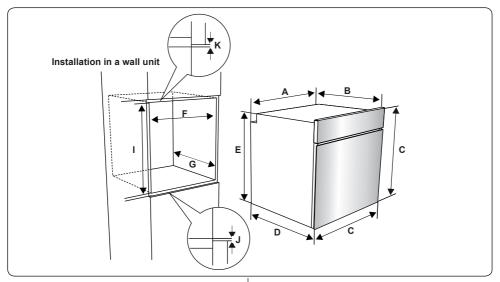
After making the electrical connections, insert the oven into the joinery by pushing it forward. Open the oven door and insert 2 screws in the holes located on the oven frame. While the oven frame touches the wooden surface of the joinery, tighten the screws.
