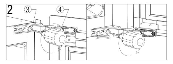
**4.** Rotate the door by 180 degrees, and install it to the other side of the cabinet. (Figure 3 and 4)
