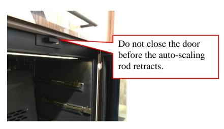
Note: In the power-off state, you cannot operate the auto-door. You can open the door from the crack directly with hand if needed.
