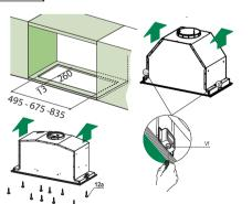
• Screw the Frame back into place using the 6 screws removed as described above, re-connect the wires to the Commands and Light, replace the metal grease filter and the Panel.
